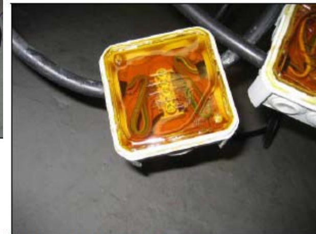
Test sample 2 after 1000h in water
