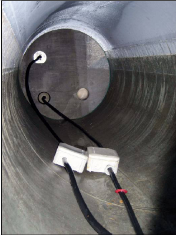
Test samples inside opened pressure tank
