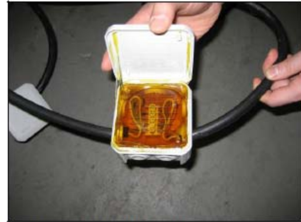
Test sample 1 after 1000h in water
