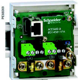
ACE949-2 2-wire RS 485 network connection interface.
