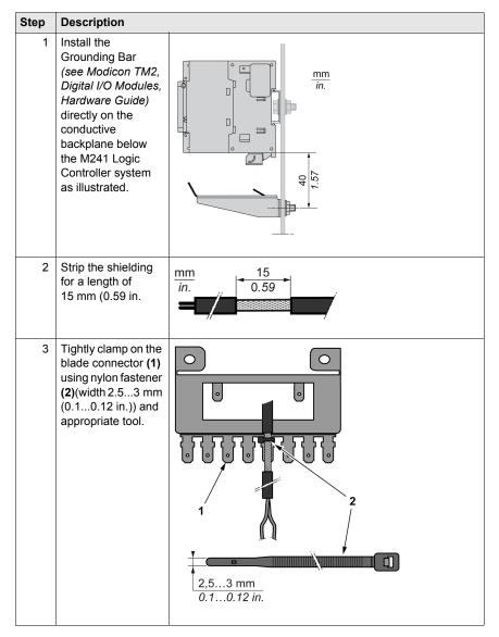
**NOTE:** Use the TM2XMTGB Grounding Bar for Functional Ground (FE) connections.
