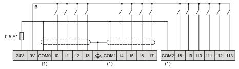
The following figure shows the source wiring (negative logic) of the controller digital inputs:
