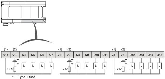
(1) The V1+, V2+ and V3+ terminals are not connected internally.
