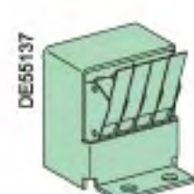
Racked in/out position
