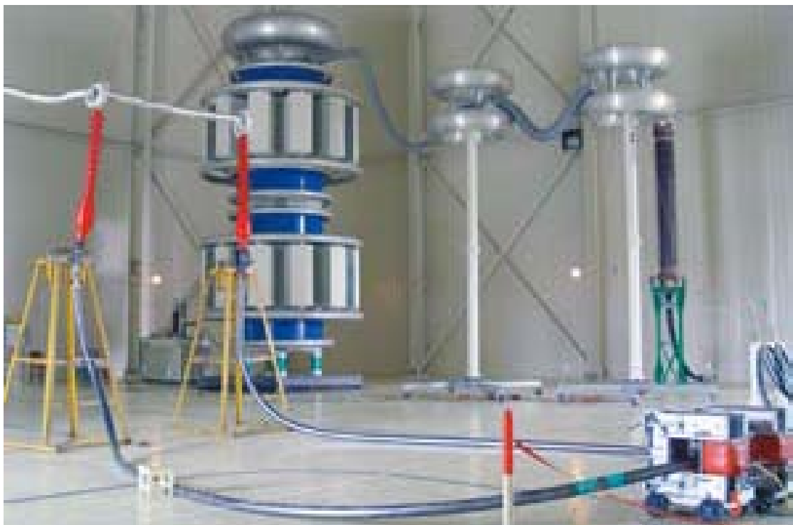
110kV dry termination is under testing in national testing center
