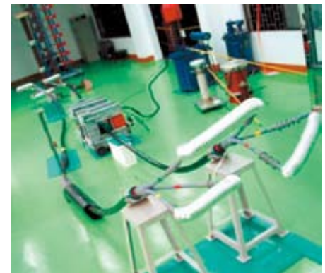
Cold shrink termination and joint are under testing
