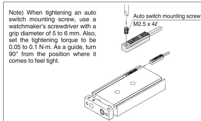
1. Insert the auto switch into the mounting groove and set it at the auto switch mounting position.
