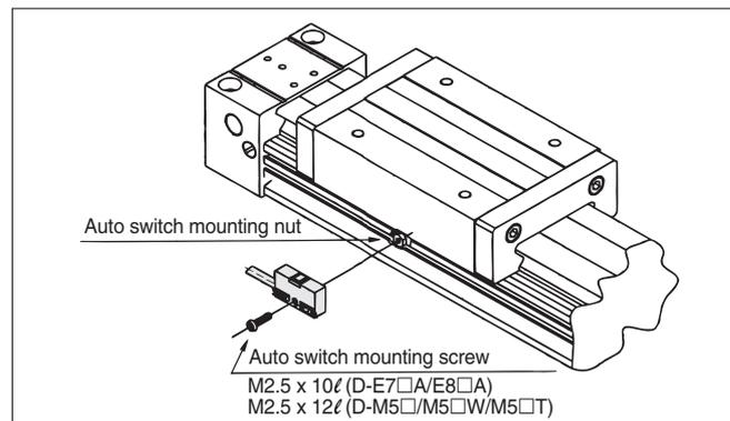
1. Insert the auto switch mounting nut into the auto switch mounting groove and then set the switch at the mounting position by sliding.
