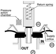
Fluid from the IN side goes through the supply orifice and fills the pressure action chamber.
